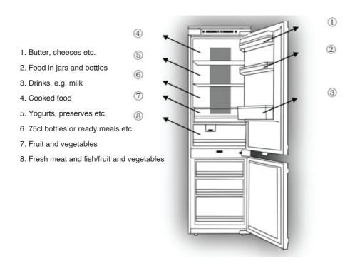
The fridge shelves can be moved according to the storage requirements within the fridge section. To move the shelf, lift up the rear section and then pull it outwards.
