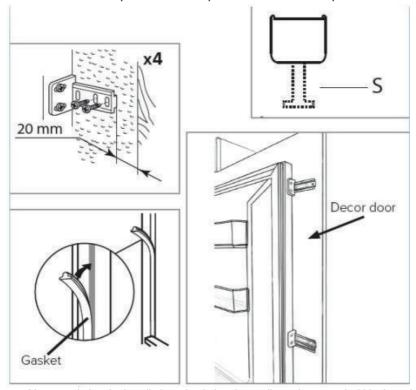
Important: After completing the installation, check that the appliance is secured within the unit and that the door(s) close and open properly. Ifthere is no resistance from the door seals when opening the doors, then it is probable that the appliance and/or decor doors are not fitted properly.
