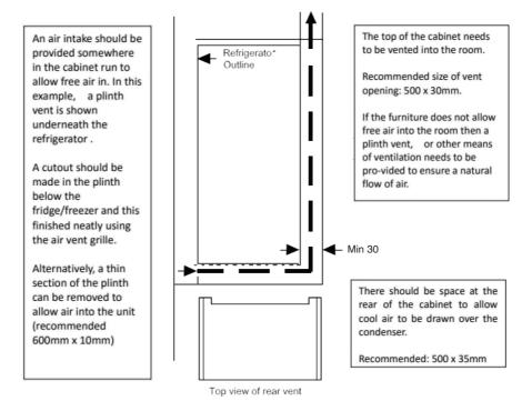
The open channel at the rear is clearly shown. For the correct operation of the appliance it is important that the top of the housing unit is notblocked off. A channel depth of 40-50mm is normal with most units.
